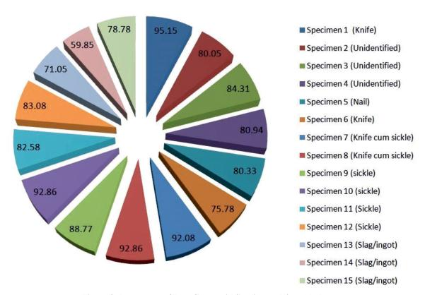
Figure 3: Percentage of Iron Content in Specimens, Niramakulam
